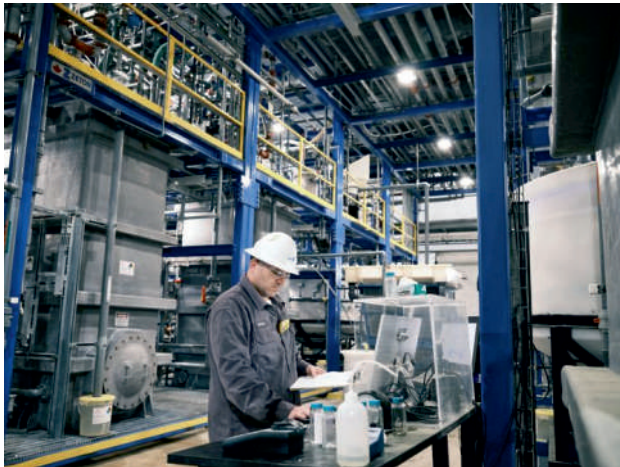
An operator at Standard Lithium monitors the performance of the continuous direct lithium extraction process and does quality-control testing on the plant floor.
